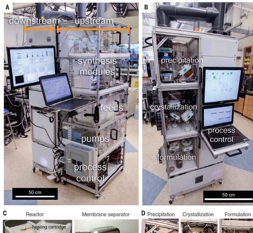
Fig. 1. Reconfigurable system for continuous production and formulation of APIs. (A) Labeled photograph of the stack of upstream synthesis modules. (B) Labeled photograph of the downstream purification and formulation modules. (C) Close-up examples of upstream units; PFA tube flow reactors in an aluminum shell for heating (left) and membrane surface tension-based separation units (right). (D) Images of some of the main components in the downstream unit including the (a) buffer tank, (b) precipitation tank, (c) filtration unit, (d) crystallization unit, (e) filtration unit, (f) formulation tank, (g) solution holding tank, and (h) formulated API. Details are in the supplementary text.
