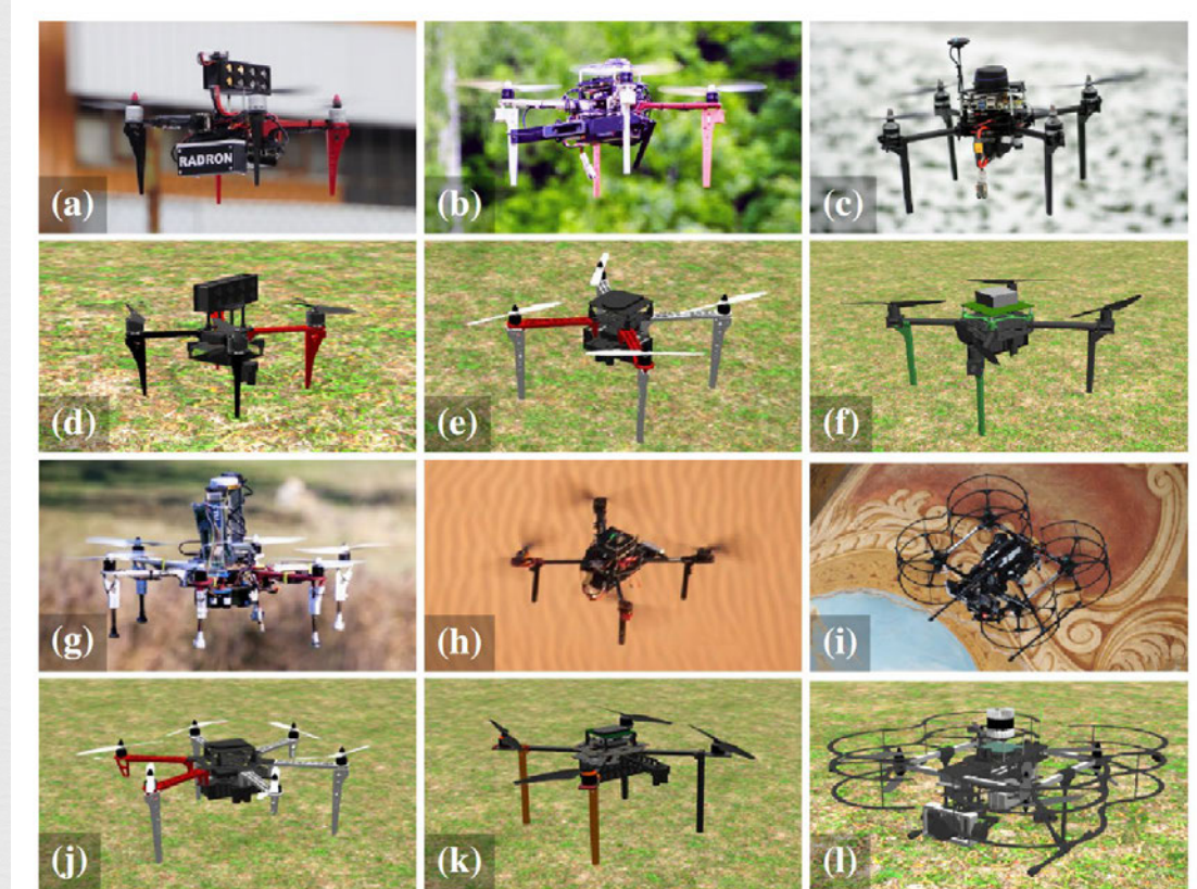
Fig. 1: MRS UAV platforms used for a diverse range of real-world applications (a)-(c), (g)-(i) and their simulated variants (d)-(f), (j)-(l), respectively. The numerous applications, ranging from aerial indoor inspection to multi-robot wall building, is enabled thanks to the high modularity of the MRS drone.
